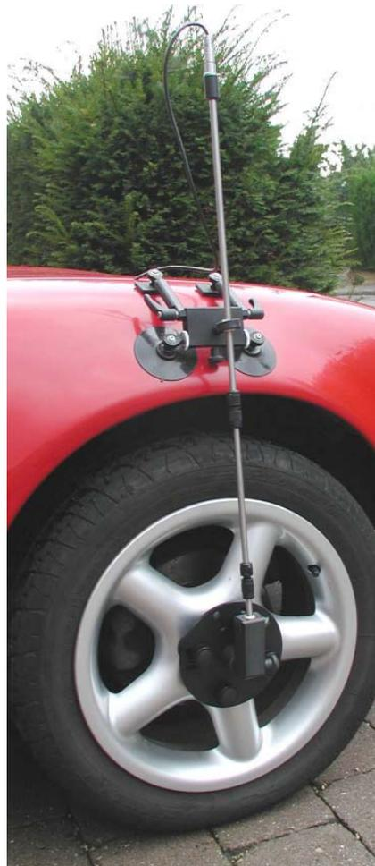
The **Clamps** main property is its high holding force. It allows attachment of heavy equipment securely to the wheel nuts, even on extremely bad roads.
